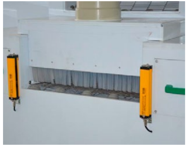
At the entrance to install safety grating
