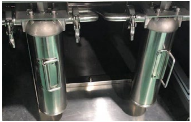
0.22um precision Filtering System ensure cleaning quality
